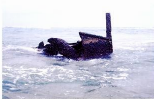
Figure 8: View of bow section of the Fiona. Note anchor hawse pipes and stem post. Photo: Tim Smith
