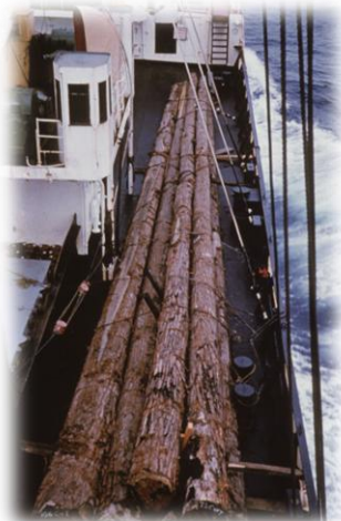
Out going turpentine wharf piles for Fiji
